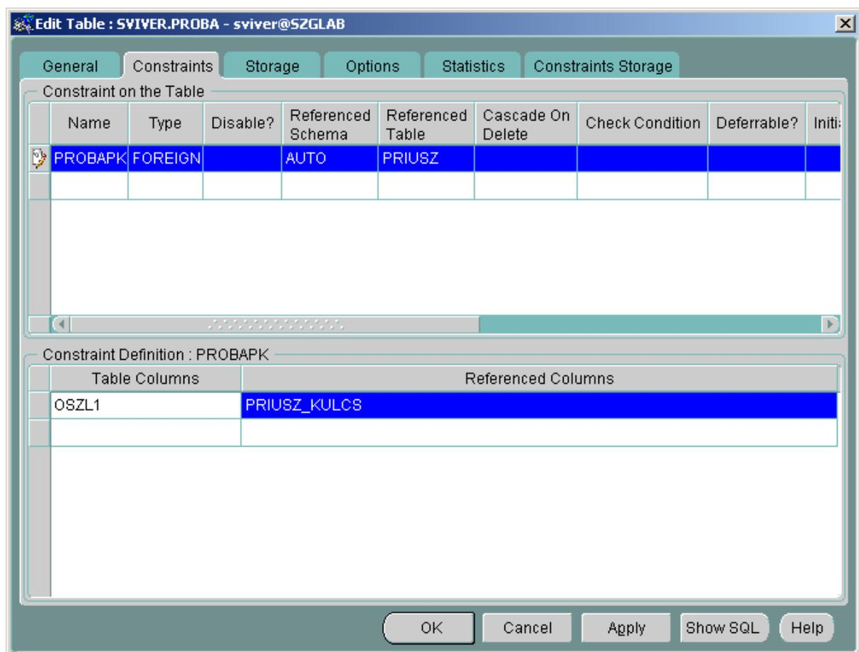
In the Enterprise Manager the Constraints tab is practically divided into two parts. The upper part (Constraint on the Table) is used to define the constraints, while the lower part is used to define the mapping between the actual constraint and the table columns (Constraint Definition). The contents of the lower part are always related to one entry in the upper part, thus upon entering data in the lower part the user must pay attention to select the appropriate constraint in the upper part.
